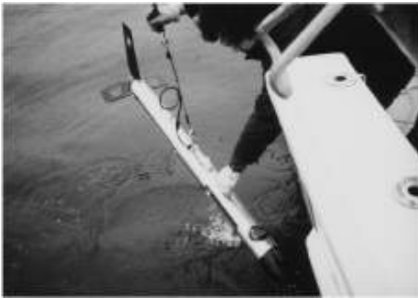
Fig. 13. Photo showing towing transducer of side-scan sonar (Komatsu et al. 2003b).
